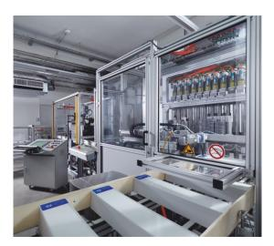
Depending on the degree of automation, an output of up to 400 pairs (800 plates) per hour can be realised with one operator only.
